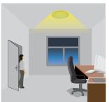
With insufficient natural light, the sensor switches on the light automatically when person enters the room. The lamp never switch off with presence, even the natural light is sufficient.
