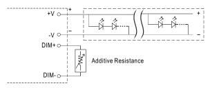
"DO NOT connect "DIM- to -V"
