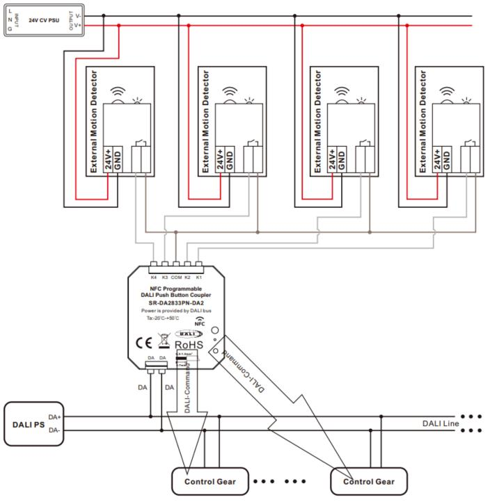
**Note:** the external motion detector can be either DC powered or AC powered, as long as its output is potential free dry contact output.
