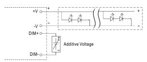
"DO NOT connect "DIM- to -V"
