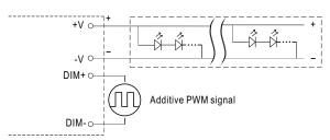
"DO NOT connect "DIM- to -V"
