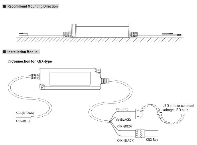
PWM KN series can be ETS adressing/programming WITHOUT connecting to AC mains
