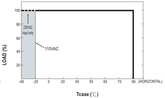
⊙ If ELG-240 operates in Constant Current mode with the rated current, the maximum workable Ta is 60°C.
