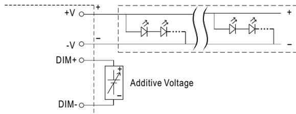
"DO NOT connect "DIM- to -V"
