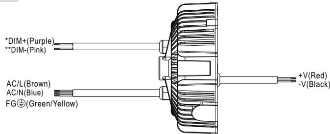
※ 3 in 1 dimming function (for B/AB-Type)
