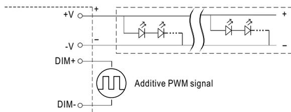
"DO NOT connect "DIM- to -V"
