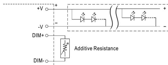
"DO NOT connect "DIM- to -V"
