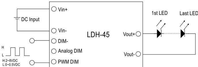
During PWM dimming operation, I<sub>O</sub> will change with the PWM duty (PWM Signal: 1K~10KHz)
