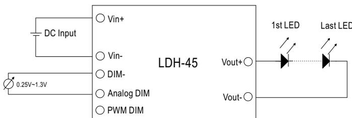
During analog dimming operation, I<sub>O</sub> will change with DC input voltage
