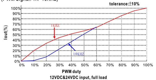
Note: DALI dimming curve refer to 10KHz curve
