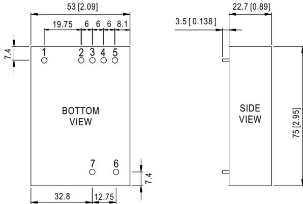
NOTE: PIN size tolerance 1.0  $\phi$   $\pm$ 0.05mm
