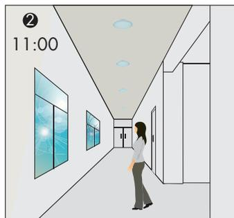
The light turns off completely whenever natural light reaches above pre-set daylight threshold.
