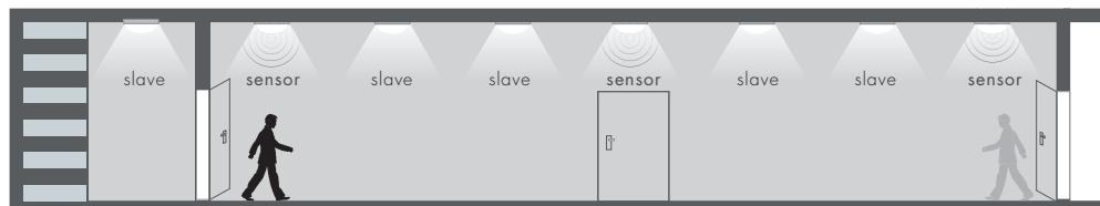
The lights dim to stand-by level after hold-time, or turn off completely if surrounding natural light is sufficient.
