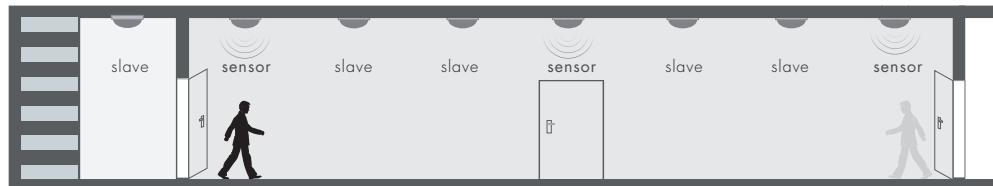
With insufficient natural light, the person comes from any direction, the whole group of lights switch on.
