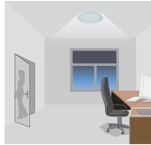
After hold-time, the light dims to light stand-by level.
