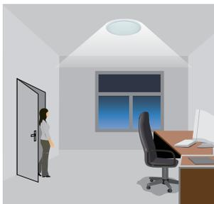
The sensor switches on the light automatically when presence is detected. The period of time the light is held on is controlled by the external sensor
