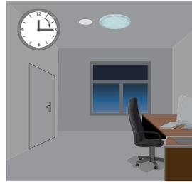
The light switches off completely after hold-time.
