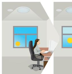
The light turns on at full or dims to maintain the lux level. The light output regulates according to the level of natural light available.
