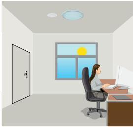
The light dims down and eventually turns off when the ambient natural light is sufficient.
