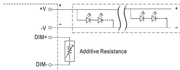
“DO NOT connect "DIM- to -V"”
