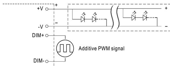
“DO NOT connect "DIM- to -V"”
