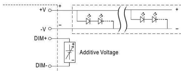
“DO NOT connect "DIM- to -V"”
