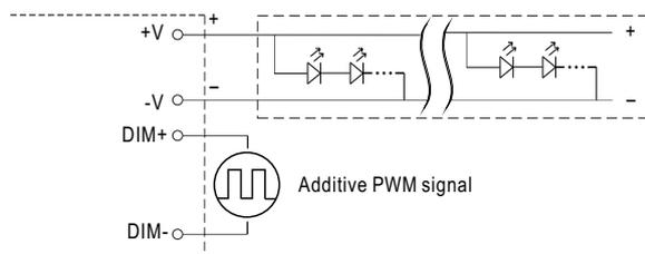
"DO NOT connect "DIM- to -V"
