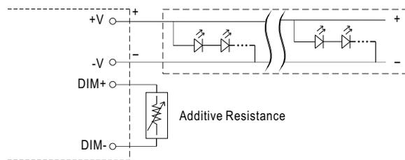
"DO NOT connect "DIM- to -V"
