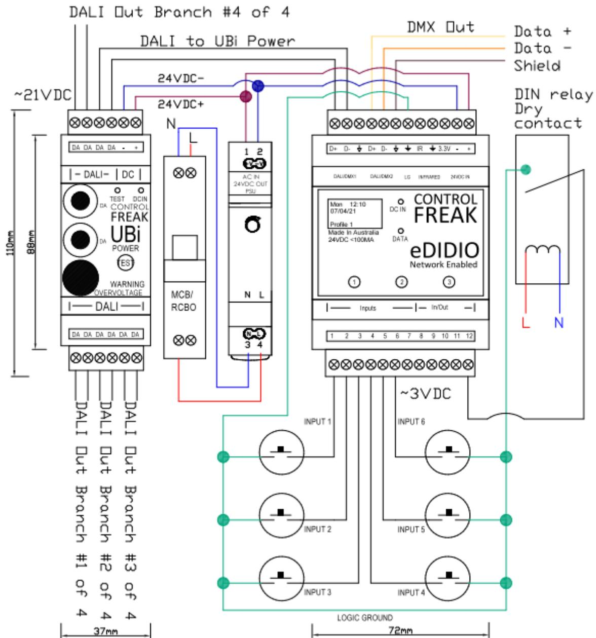
Figure 1. Example Wiring diagram showing DMX<sub>512-A</sub> and DALI. Also depicts examples of connecting I/Os for switches, relays et cetera
