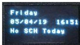
An information line is available at the bottom of the display which will provide status updates on either; Schedules, Burn-in, or current profile. The default is schedule status and is settable using the keypad menu.
