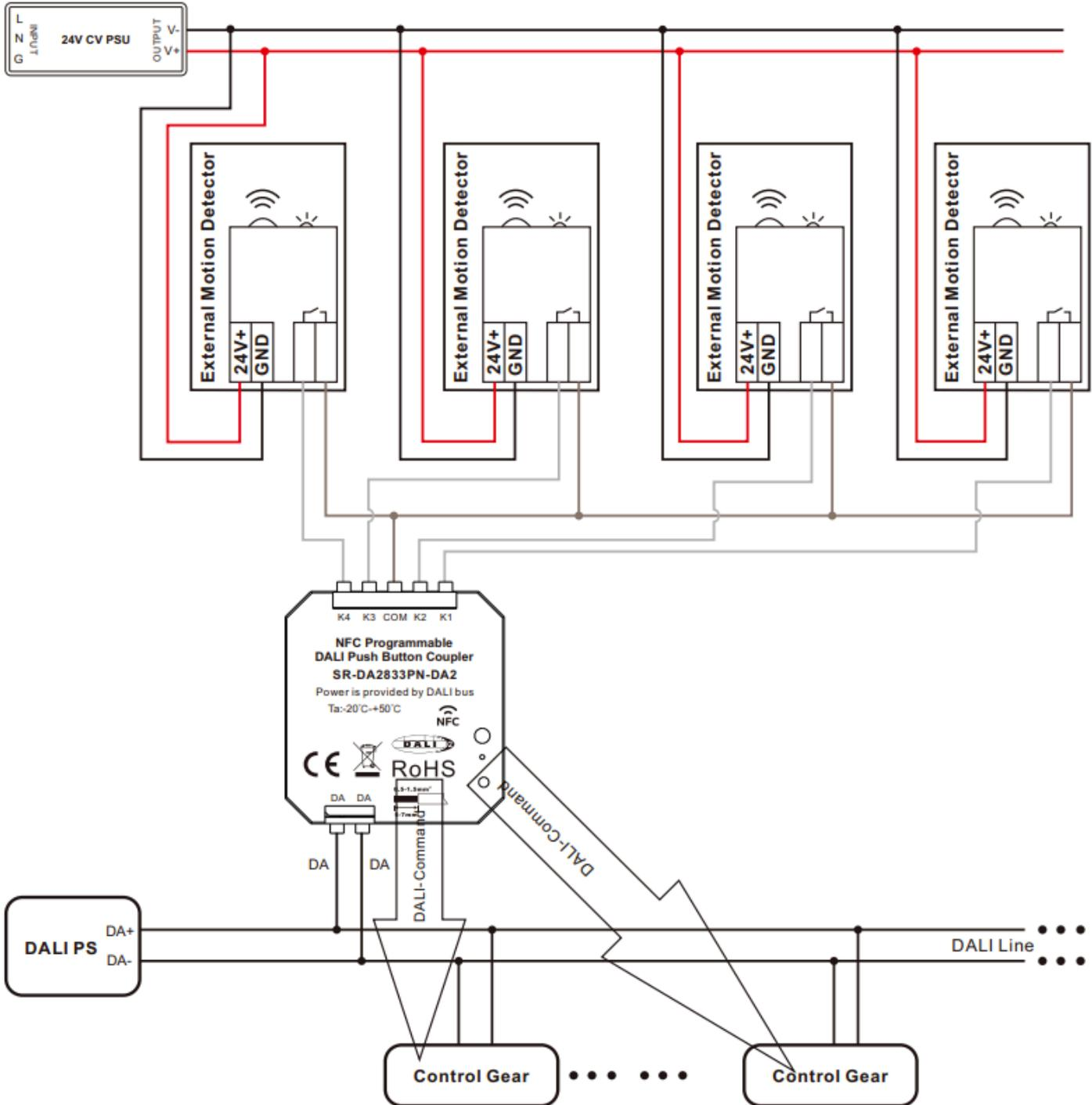
**Note:** the external motion detector can be either DC powered or AC powered, as long as its output is potential free dry contact output.
