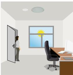
Light will not switch on when natural light is sufficient, even there is motion detected.
