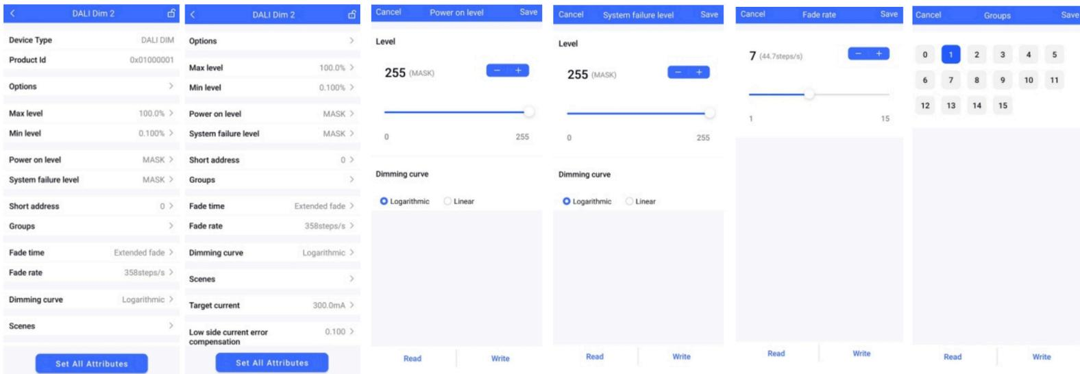
Step 5: After setting, please save the selected configuration via NFC and power on the device
