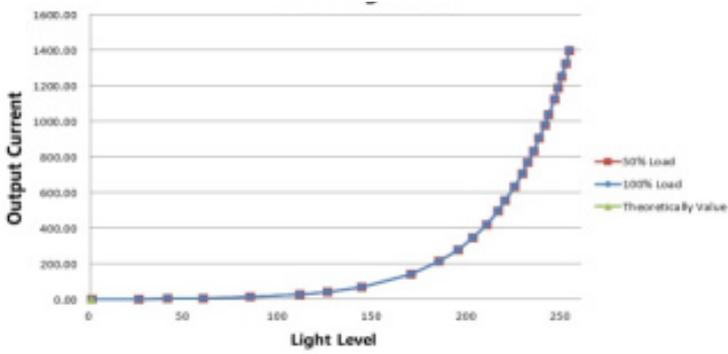
Note: Test data under 1400mA gear
