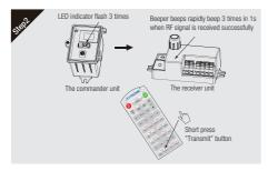
Short press "Transmit" button on RC to the commander, the red indicator on commander unit will flash 3 times to send the transmission signal.
