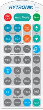
Note: the buzzer beeps one time when RC receives signal successfully.
