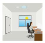
The light switches off when the ambient natural light is sufficient.
