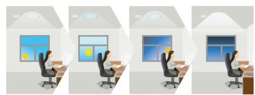
The light turns on at full or dims to maintain the lux level. The light output regulates accroding to the level of natural light available.
