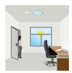
Light will not switch on when natural light is sufficient, even there is motion detected.
