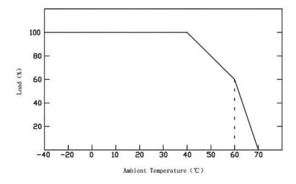
If being used in higher ambient temperatures, ensure the load on the LED driver is de-rated in accordance with this chart. Failure to do so could lead to a premature failure, which is not covered by the warranty.
