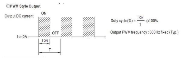
When the "On" period equates to 50% of the duty cycle, as it does in the above diagram, the light level will be at 50% of maximum brightness. If the "On" period equates to 100% of the duty cycle the lights would be at maximum brightness.
