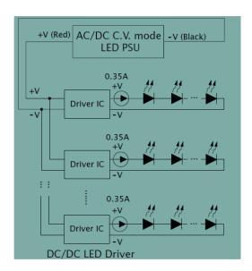
Each string of LEDs is driven by a driver giving a constant current output. These drivers are supplied from a constant voltage power supply. It gives more accurate control over each string and single LED failure can be easily controlled. It offers flexible design particularly with multi strips.
