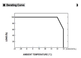
In this example the derating curve shows at 60 degrees Celsius the maximum load on the driver should be limited to 60% of its maximum rated capacity. It is important to check the derating curve, as it may be necessary to use a larger capacity LED driver than originally anticipated.
