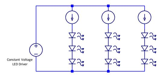
Direct drive architecture can be prone to imbalance if there is one LED drawing a bit more current than it should, or if one has failed completely. Using IC type drivers will prevent this problem but incurs a higher cost.
