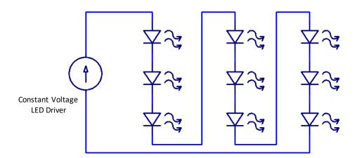
Firstly, for very long strings the brightness of the LEDs gets dimmer the further down the string they are. This is because each LED adds a little resistance to the circuit. Under normal circumstances it is not enough to affect the performance of the LEDs. But the aggregate resistance in a long string can cause a voltage drop to make enough of a difference to effect the function of an LED.
