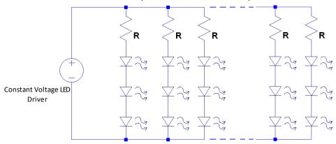
It has a low level of complexity and is a low-cost solution. However, it has poor current regulation and low efficiency.
