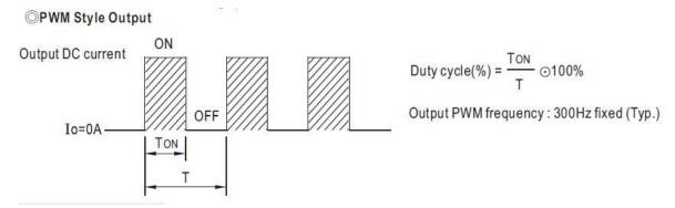
When the "On" period equates to 50% of the duty cycle, as it does in the above diagram, the light level will be at 50% of maximum brightness. If the "On" period equates to 100% of the duty cycle the lights would be at maximum brightness.
