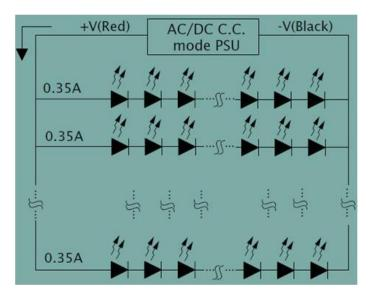
Again it has a low level of complexity, but a high level of efficiency. It is also a low-cost solution. As previously mentioned, it is prone to current imbalance. For example, if you have one LED drawing more current it could result in a voltage drop on that string, altering the brightness of the LEDs. This architecture is also vulnerable should a single LED fail.
